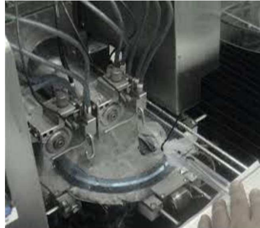
Figure 1. Wafer Saw Process with ESD Sensor
