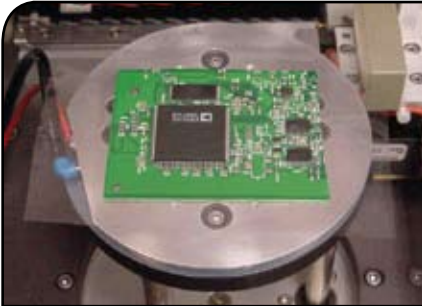
Figure 1: FICBM test method setup for a DSP board. After Olney [9].
